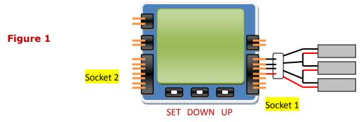
2. For two battery packs, connect them in series first and then plug battery 1# into socket 1, and battery 2# into socket 2 separately. Take 2 3s battery sample as following:
