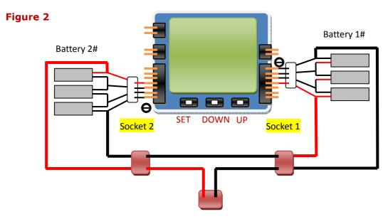
Socket1 and socket2 can deal up to 6S battery independently, so you can connect any combo battery pack on condition that the total cell count less than 12, such as 6S+6S, 2S+6S, 5S+6S, 6S+3S, 6S+5S and so on.
